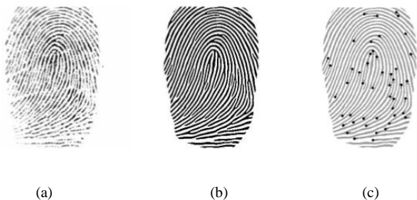
Fig. 7. Feature Extraction Process (a) original (b) after process (c) along with feature points
