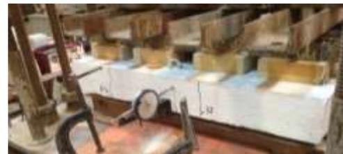
Figure (5): Horizontal dial gauges for slippage measurements.
