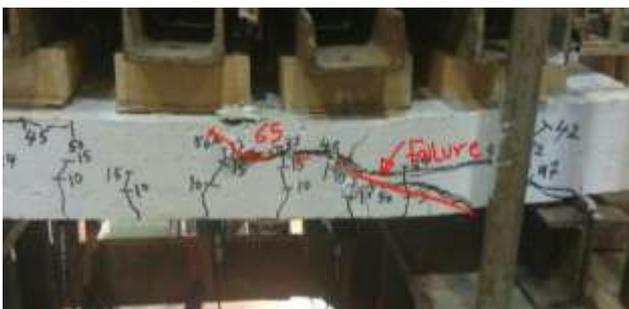
Figure (9): Shear failure of slab S2.
