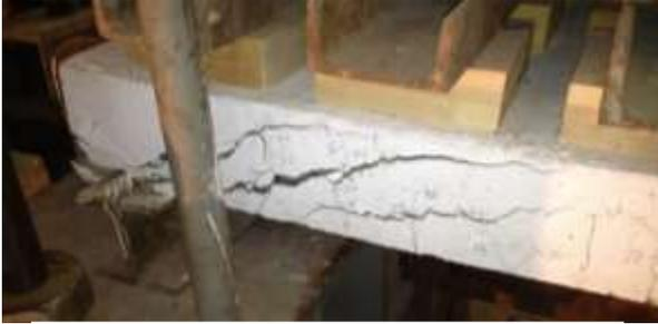
Figure(7): Shear failure of slab S1.
