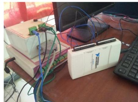
Figure 2: Interfaced NI-DAQmx 6211 Data Acquisition Module Card.
